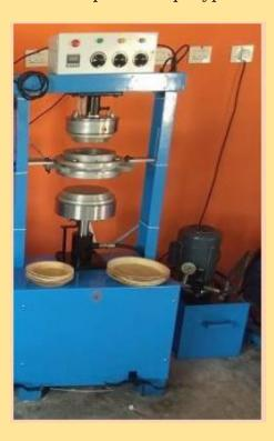
Stainless steel blades &, first grade aluminum die. 1hp motor 1phase/3phase as per your need. Total Power required: Single phase line with 4 HP = 3 KW = 3000 WATTS Output: 1 operator 80 plates per hour and around 640 in 8 hours.
